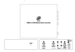
A general overview drawing of the VS-226 shows the input and output connectors and controls.
